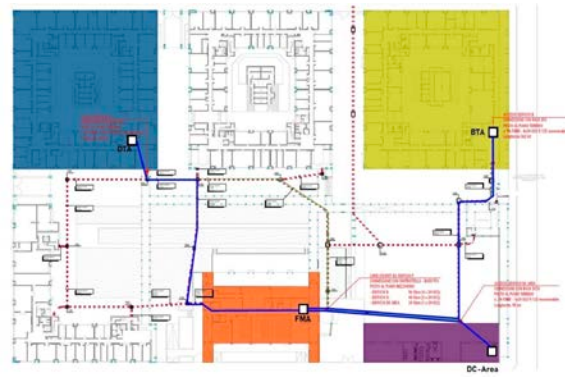
Scheme of the CNR Research Area of Firenze with the external fibre-optic backbone (blue lines) connecting building "F" (core) and buildings "B", "D" e "DC-Area".
